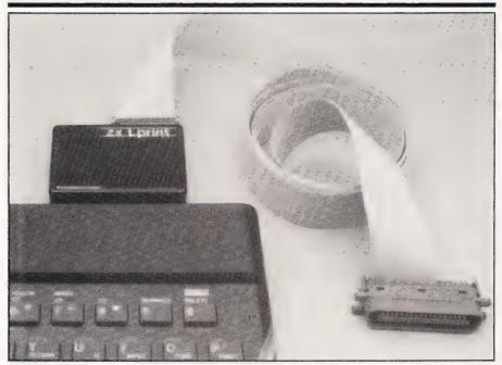
the ZX Spectrum computer it was promoted as a machine for games and learning about computers. Since then it has found use as a business planner, a filing system and even as a word-processor. The system was designed to work with only one printer — the cheap but restricted ZX printer made by Sinclair. Unlike other home computers the Spectrum does not contain the necessary interface electronics to allow it to be connected to a more sophisticated printer.
